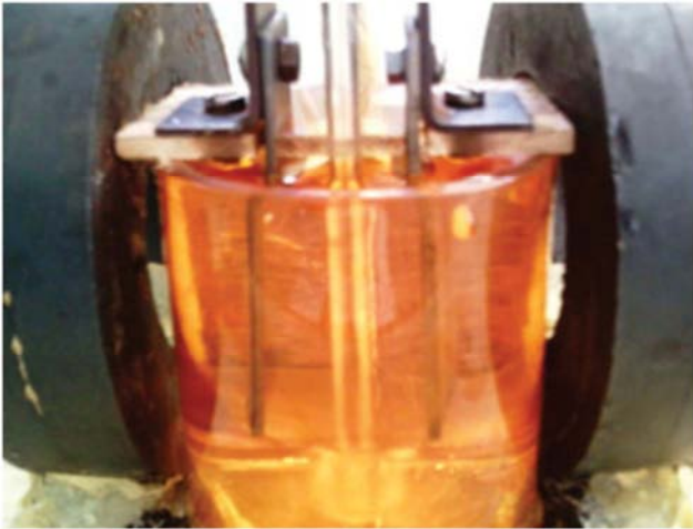
Figure 3. The apparatus of EC with MF magnets placed for the treatment of MO [29].
